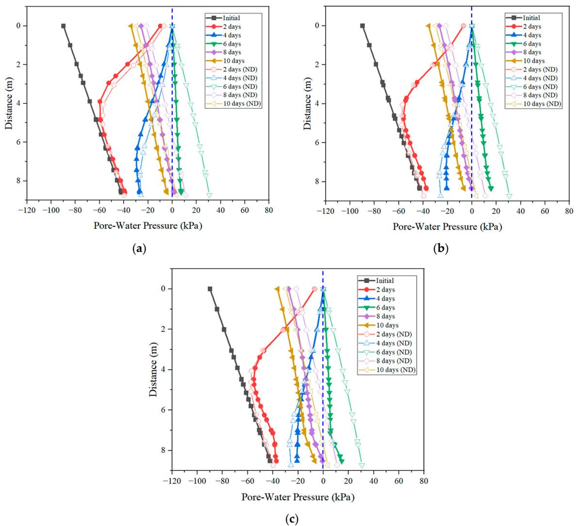
Figure 6. Impact of horizontal drain inclination angle on pore-water pressure in Section 2: (a) 5° horizontal drain; (b) 10° horizontal drain; (c) 15° horizontal drain.
