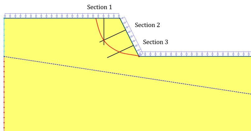
**Figure 2.** Positioning of the varying analysis sections within the slope.
