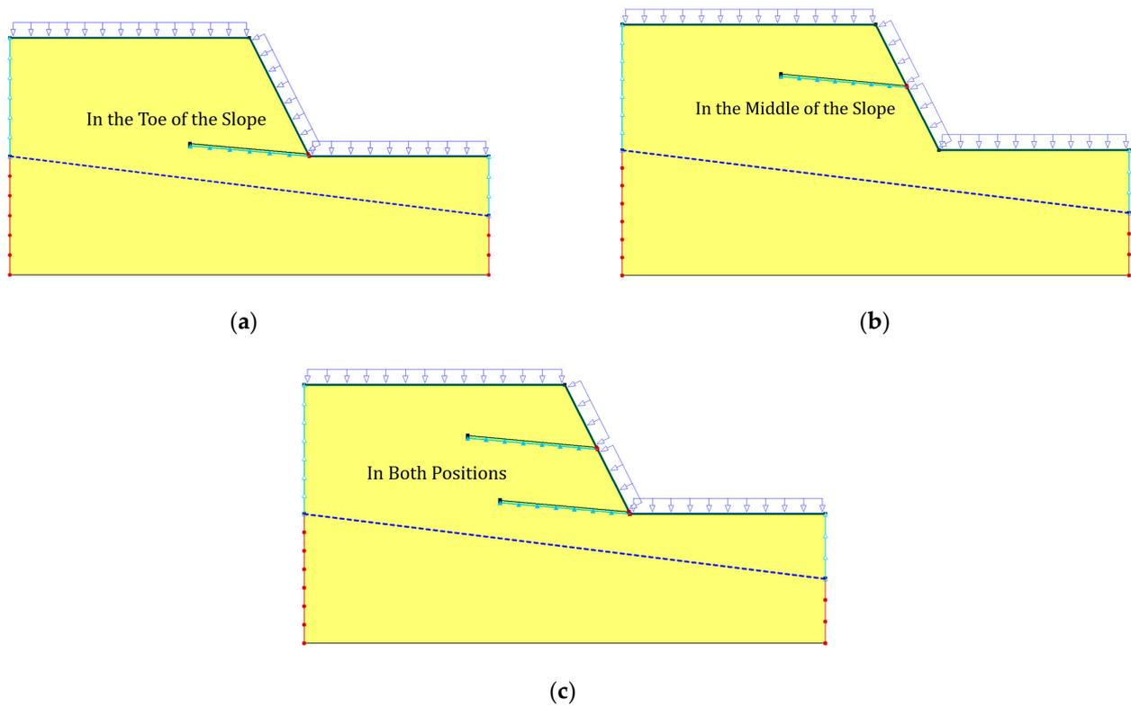
**Figure 8.** Displacement position of horizontal drains: (a) at the toe of the slope; (b) at the middle of the slope; (c) in both positions.
