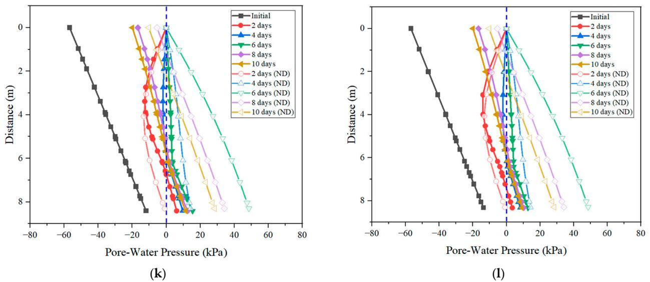
**Figure 4.** Impact of horizontal drain length on pore-water pressure in slopes: (a–d) comparison of 4 m, 7 m, 10 m, and 13 m in Section 1; (e–h) comparison of 4 m, 7 m, 10 m, and 13 m in Section 2; (i–l) comparison of 4 m, 7 m, 10 m, and 13 m in Section 3.
