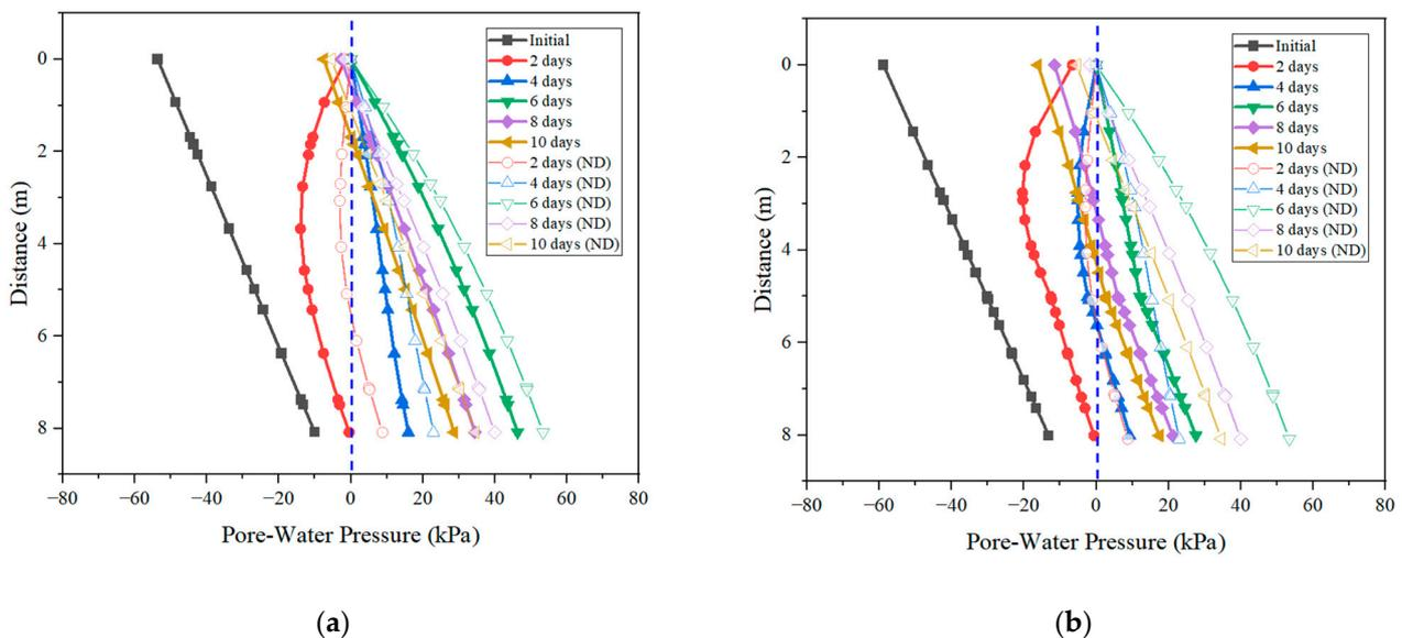
**Figure 11.** Impact of horizontal drain placement position on pore-water pressure in Section 3: (a) at the middle of the slope; (b) at both positions.
