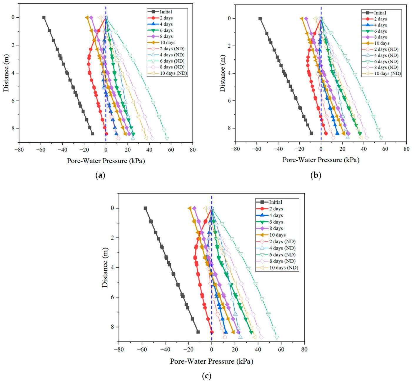
**Figure 7.** Impact of horizontal drain inclination angle on pore-water pressure in Section 3: (a) 5° horizontal drain; (b) 10° horizontal drain; (c) 15° horizontal drain.
