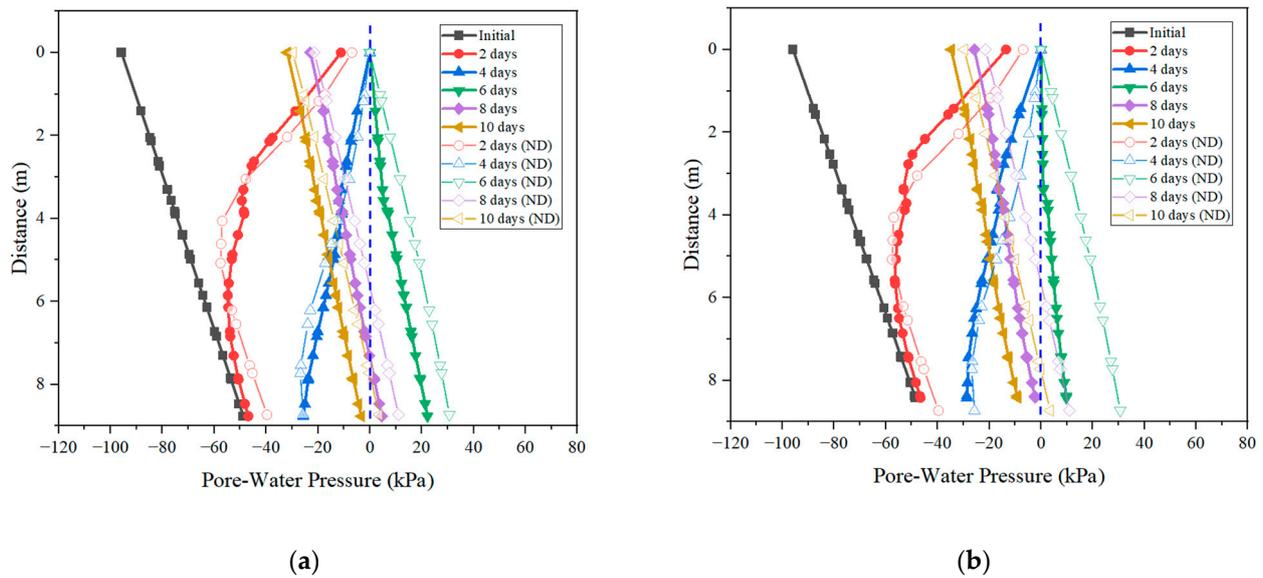
**Figure 10.** Impact of horizontal drain placement position on pore-water pressure in Section 2: (a) at the middle of the slope; (b) at both positions.
