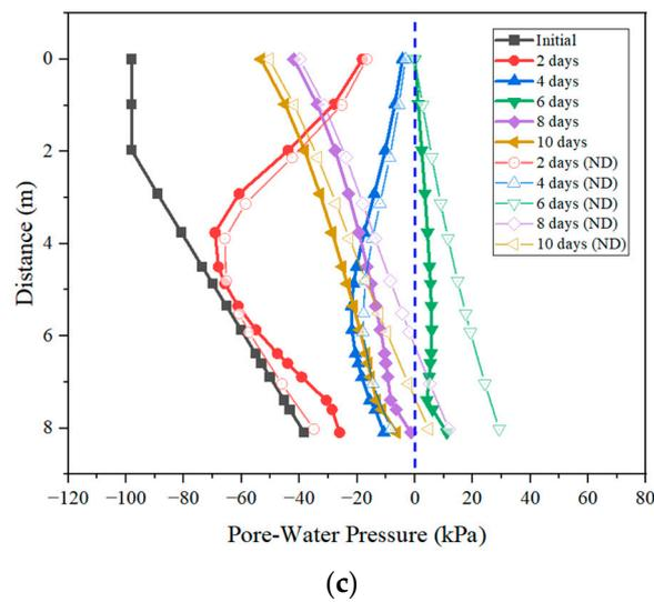
Figure 5. Impact of horizontal drain inclination angle on pore-water pressure in Section 1: (a) 5° horizontal drain; (b) 10° horizontal drain; (c) 15° horizontal drain.
