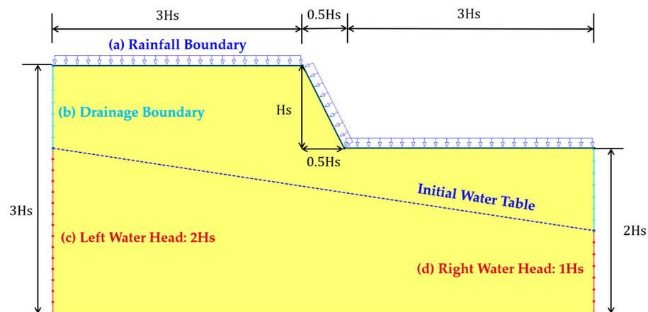
**Figure 1.** Geometric and boundary conditions of the numerical model.
