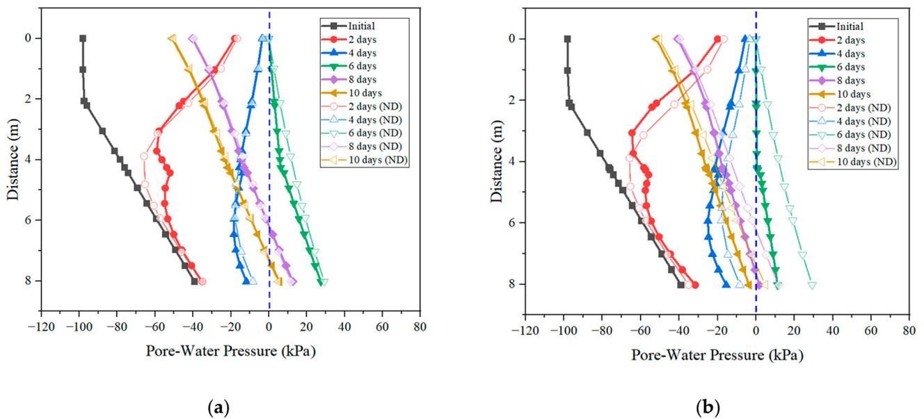
**Figure 9.** Impact of horizontal drain placement position on pore-water pressure in Section 1: (a) at the middle of the slope; (b) at both positions.
