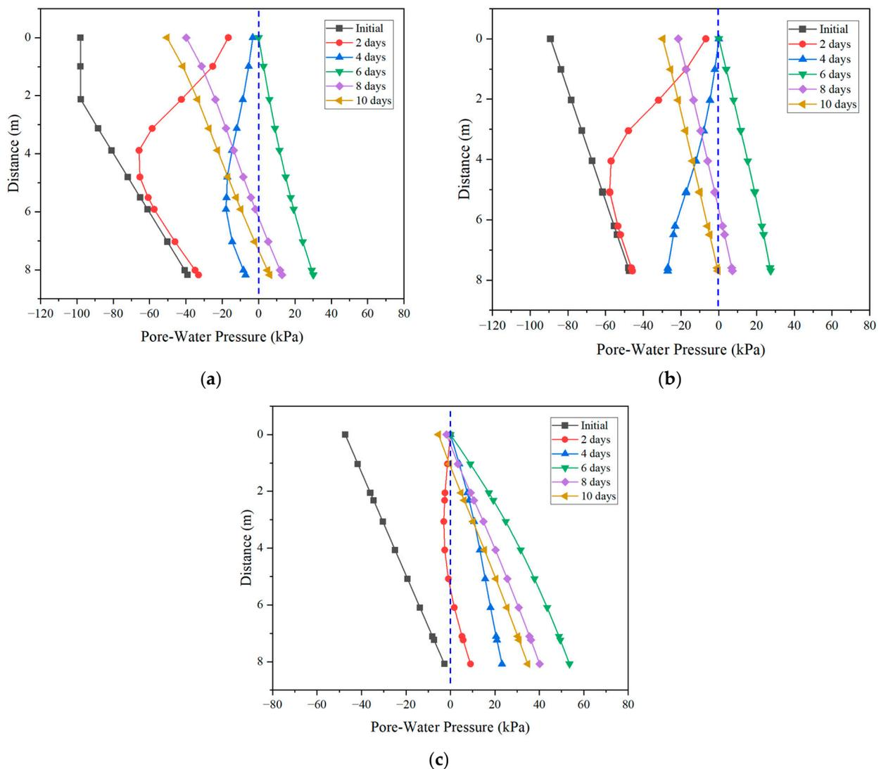
**Figure 3.** Pore-water pressure distribution across three sections of the slope under no-drainage condition: (a) Section 1; (b) Section 2; (c) Section 3.
